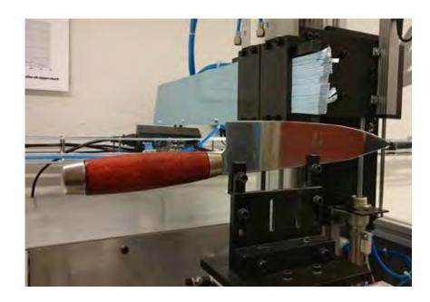
Many of our knives needs to be flexible. This mainly applies to our wide range of food processing knives, but all our models need to have strong and reliable blades. The laboratory allows us to test and evaluate the bending force, so that we can ensure that the way we treat the steel - according to our SGM® (Steel Grade Mora) standard - is as well functioning as ever.
